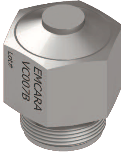
CONNECTION: ACCEPTS PRE-SWAGED 3 4 TUBE WITH NUT AND FERRULE NOMINAL CRACKING PRESSURE: 10 - 20 PSI
