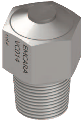
CONNECTION: THREADS DIRECTLY INTO 3 4" NPT FITTING NOMINAL CRACKING PRESSURE: 10 - 20 PSI
