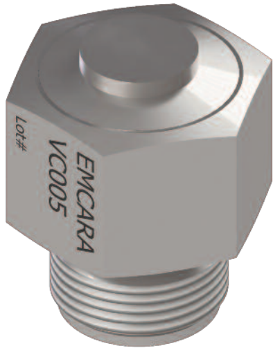
CONNECTION: ACCEPTS PRE-SWAGED 1 2" TUBE WITH NUT AND FERRULE NOMINAL CRACKING PRESSURE: 10 - 20 PSI
