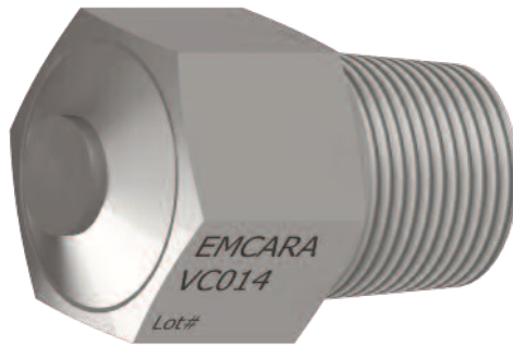
CONNECTION: THREADS DIRECTLY INTO 3/4" NPT FITTING NOMINAL CRACKING PRESSURE: 10 - 20 PSI
